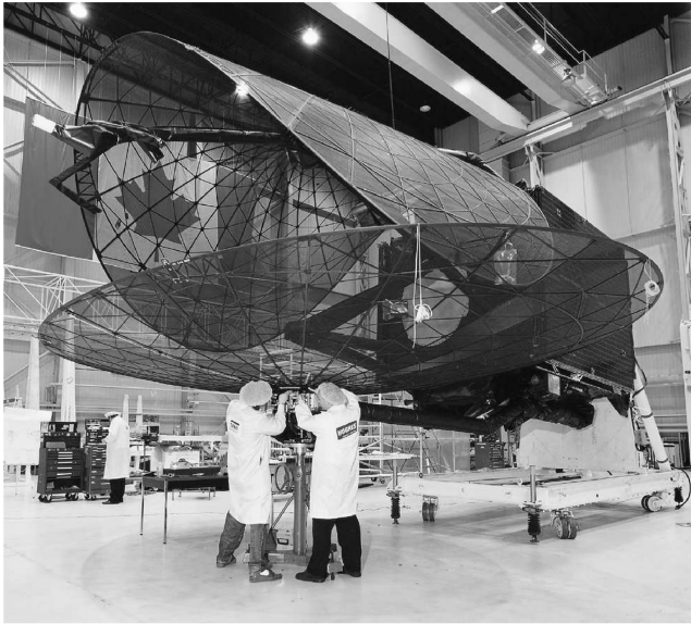
Fig. 1 MSAT-2 spacecraft during ground testing with two spring back reflectors, one deployed and one folded. Courtesy: Communications Research Centre (CRC), Industry Canada.
